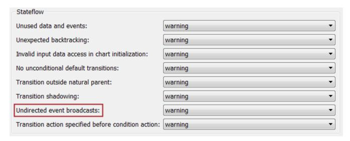
Undirected local event broadcasts can cause unwanted recursive behavior in a chart and inefficient code generation. You can avoid this behavior by using the send operator to create *directed* local event broadcasts. For more information, see Guidelines for Avoiding Unwanted Recursion in a Chart and Broadcasting Events to Synchronize States.
